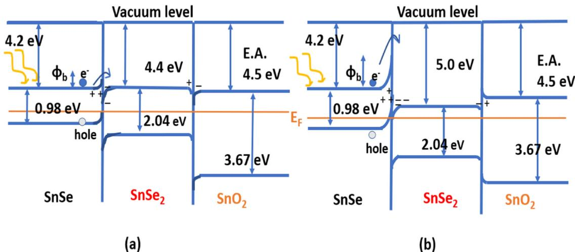
Fig. 6 Schematic diagram of the band alignment of the configuration when the E.A. of SnSe<sub>2</sub> is (a) 4.4 eV and (b) 5.0 eV. E.A. (5.0 eV) makes the barrier a greater height and creates a potential well in the transportation of the carriers.
