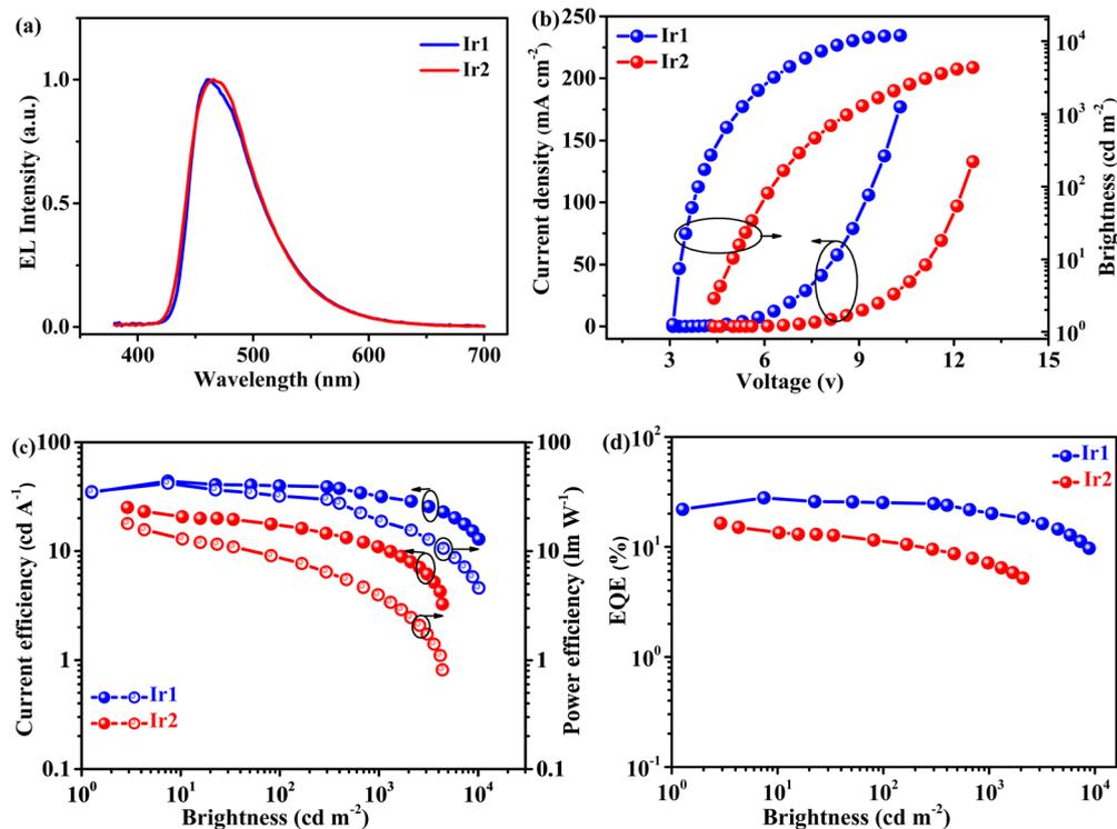
Fig. 6 The performance of devices based on complexes **Ir1** and **Ir2**: (a) EL spectra, (b) current density–voltage–brightness ( $J$ – $V$ – $B$ ) characteristics, and (c) CE and PE vs luminance curves and (d) EQE–luminance curves.
