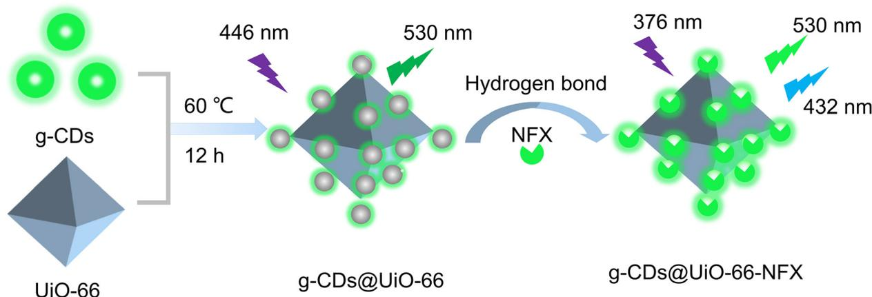
Scheme 1 Schematic representation for the preparation of g-CDs@UiO-66 and its application in norfloxacin sensing.
