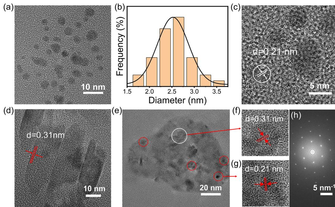
**Fig. 1** (a) TEM and (c) HRTEM images of g-CDs. (b) Size distribution of the g-CDs. (d) HRTEM image of UiO-66. (e) TEM and (f and g) HRTEM images of g-CDs@UiO-66. (h) SAED pattern of g-CDs@UiO-66.
