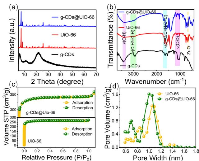
**Fig. 2** (a) XRD patterns of the g-CDs (black line), UiO-66 (red line), and g-CDs@UiO-66 (blue line). (b) FT-IR spectra of the g-CDs, UiO-66, and g-CDs@UiO-66. (c) N<sub>2</sub> adsorption–desorption isotherms, and (d) pore volume distributions of UiO-66 and g-CDs@UiO-66.
