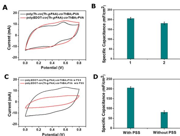
Fig. 2 (A) Cyclic voltammograms (CVs) and (B) areal specific capacitances of (1) poly(EDOT-co-(Th-g-PAA)-co-ThBA)-PVA hydrogels and (2) poly(Th-co-(Th-g-PAA)-co-ThBA)-PVA hydrogel electrodes in 2 M KCl solution at a scan rate of 100 mV s<sup>-1</sup>. (C) CV and (D) areal specific capacitance of poly(EDOT-co-(Th-g-PAA)-co-ThBA)-PVA hydrogels with and without PSS.
