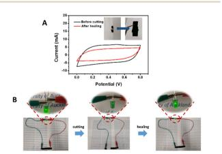
Fig. 6 (A) CV measurements of the device before cutting and after selfhealing. Inset: The photographs showing the device before cutting and after healing. (B) The green LEDs were lighted up after a cutting-healing cycle.
