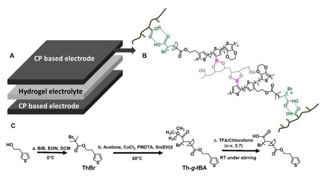
Fig. 1 (A) The "sandwich" structure of the supercapacitor. (B) The chemical structure of the poly(EDOT-co-(Th-g-PAA)-co-ThBA)-PVA hydrogel. (C) Synthetic route to Th-g-PAA.
