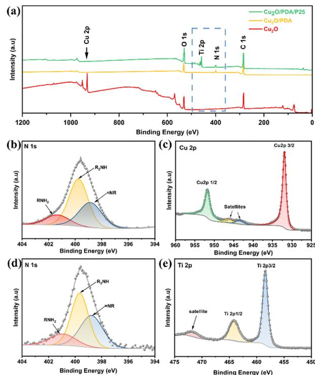
Fig. 2 (a) XPS pattern full spectra of  $\text{Cu}_2\text{O}$ ,  $\text{Cu}_2\text{O}/\text{PDA}$  and  $\text{Cu}_2\text{O}/\text{PDA}/\text{P25}$ . (b) High-resolution XPS spectra of N 1s in  $\text{Cu}_2\text{O}/\text{PDA}$  and (c) Cu 2p in  $\text{Cu}_2\text{O}$ . (d) High-resolution XPS spectra of N 1s in  $\text{Cu}_2\text{O}/\text{PDA}/\text{P25}$  and (e) Ti 2p.
