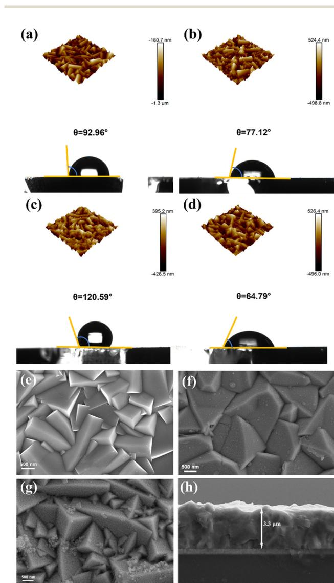
Fig. 3 AFM 3D image of a  $10 \times 10\ \mu\text{m}^2$  region and their contact angle of (a)  $\text{Cu}_2\text{O}$ , (b)  $\text{Cu}_2\text{O}/\text{PDA}$ , (c)  $\text{Cu}_2\text{O}/\text{P25}$  and (d)  $\text{Cu}_2\text{O}/\text{PDA}/\text{P25}$ . SEM image of (e)  $\text{Cu}_2\text{O}$ , (f)  $\text{Cu}_2\text{O}/\text{PDA}$ , (g)  $\text{Cu}_2\text{O}/\text{PDA}/\text{P25}$  and its side image (h).
