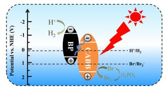
Fig. 6 Schematic illustration of the H<sub>2</sub> evolution of the BP/CABB composites
