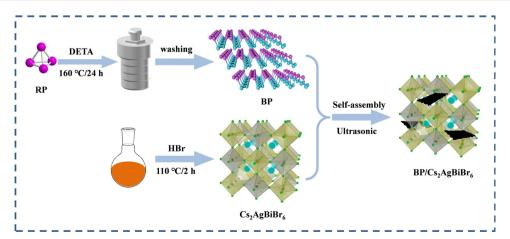
Fig. 1 Schematic diagram of the BP/CABB composite fabrication process.
