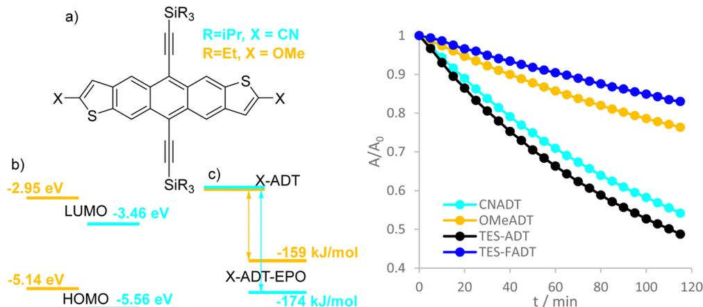
Fig. 7 (a) Structure of TES-OMeADT (orange) and TIPS-CNADT (cyan), (b) molecular orbital energies estimated from cyclic voltammetry, (c) computed reaction enthalpies for endoperoxide formation, (d) normalised absorbance of TIPS-CNADT and TES-OMeADT in  $\text{CHCl}_3$  at  $33 \mu\text{M}$  under irradiation by white LED. TES-ADT and TES-FADT (same conditions) are shown for comparison.
