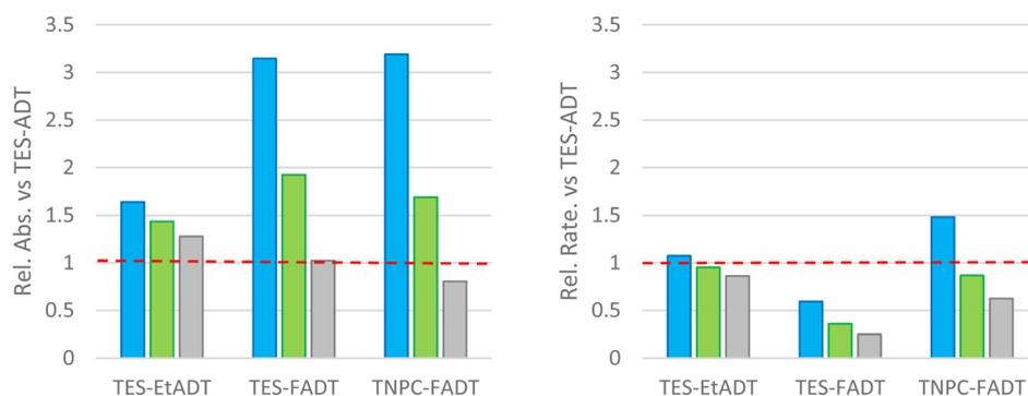
Fig. 3 (left) Integrated absorbance of ADTs *versus* light source spectra relative to the parent TES-ADT. (right) Relative reaction rates for photo-oxidation of ADTs using different coloured light sources, estimated from linear fits of absorbance over 10 minutes where  $A/A_0 > 0.9$ . All data relative to values determined for parent TES-ADT (depicted as the red line) with the same light source (blue, green, or white LED) and same concentration ( $3.3 \mu\text{M}$  in  $\text{CHCl}_3$ ).
