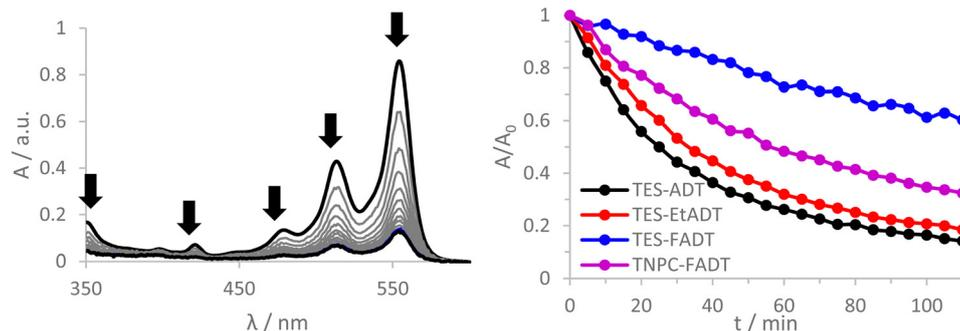
Fig. 2 (left) Absorption spectra of TES-ADT in  $\text{CHCl}_3$  measured at timed intervals while under illumination from an LED desk lamp. (right) Normalised absorbance at  $\lambda_{\text{max}}$  for ADTs over time, while under illumination from an LED desk lamp.
