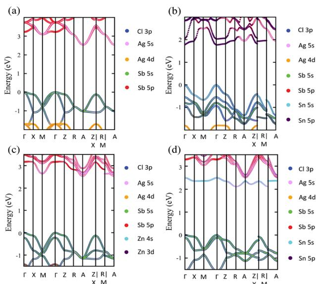
Fig. 4 Partial band structure of (a) the pristine perovskite, and the (b)  $\text{Sn}^{2+}$ - $\text{Sn}^{2+}$ , (c)  $\text{Zn}^{2+}$ - $\text{Zn}^{2+}$ , and (d)  $\text{Sn}^{4+}$ - $\text{V}_{\text{Ag}}$  doped perovskites. Color codes are added to show the orbital contributions to the bottom of the CB and the top of the VB.
