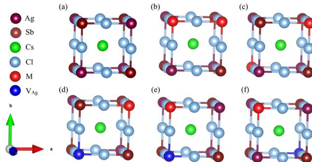
Fig. 1 Schematic models of the cubic unit of (a) the pristine  $\text{Cs}_2\text{AgSbCl}_6$  conventional cell, (b and c) configuration 1 with neighboring and distant M dopant atoms, respectively, (d) configuration 2, and (e and f) configuration 3 with a neighboring and distant M dopant atom and  $\text{V}_{\text{Ag}}$ , respectively.
