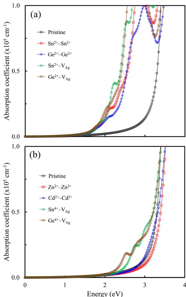
Fig. 6 (a and b) Calculated absorption coefficients of the pristine and all doped perovskites.
