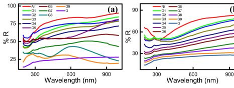
Fig. 4 Optical reflectance spectra of (a) G: Al and (b) G: Ni electrodes.
