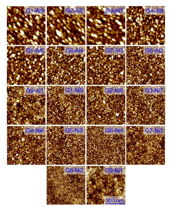
Fig. 5 Surface topography (area:  $1 \times 1 \mu m$ ) of the G: Al and G: Ni electrodes measured using AFM in noncontact mode.
