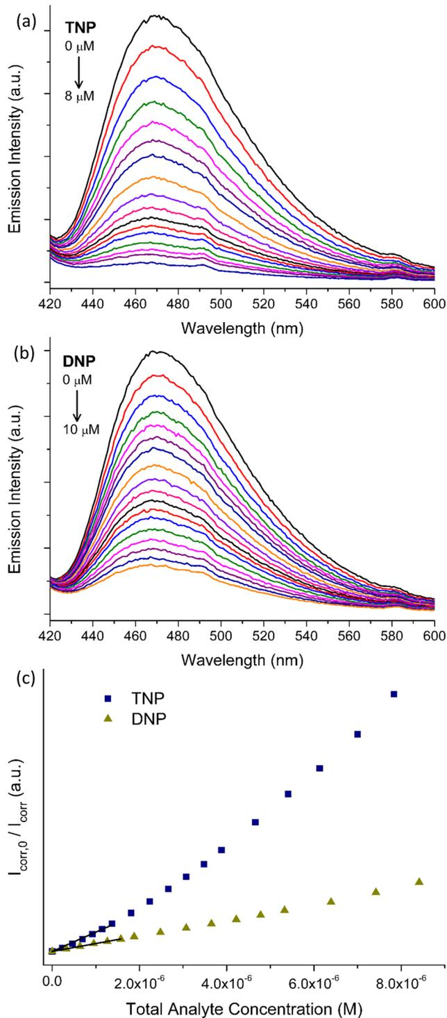
Fig. 5 Fluorescence titrations ( $\lambda_{\text{exc}} = 400 \text{ nm}$ ) of **pZr-1** suspended in H<sub>2</sub>O (2 mL, 0.1 mg mL<sup>-1</sup>) at pH 4.5 upon gradual addition of aqueous solution ( $5 \times 10^{-5} \text{ M}$ ) of (a) TNP (b) DNP (c) Corresponding Stern–Volmer plots for both titrations, showing linearity at low analyte concentrations.
