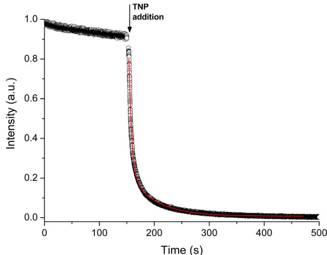
Fig. 8 Time-dependent fluorescence response ( $\lambda_{exc} = 400$  nm,  $\lambda_{em} = 470$  nm) of **pZr-1** suspended in  $H_2O$  (2 mL,  $0.1$  mg  $mL^{-1}$ ) at pH 4.5 upon addition of 25  $\mu L$  an aqueous solution of TNP ( $10^{-3}$  M). The concentration of TNP corresponds to that at the end of a typical titration experiment (8  $\mu M$ ). Black circles represent experimental data, the red curve represents the best fit based on a biexponential decay.
