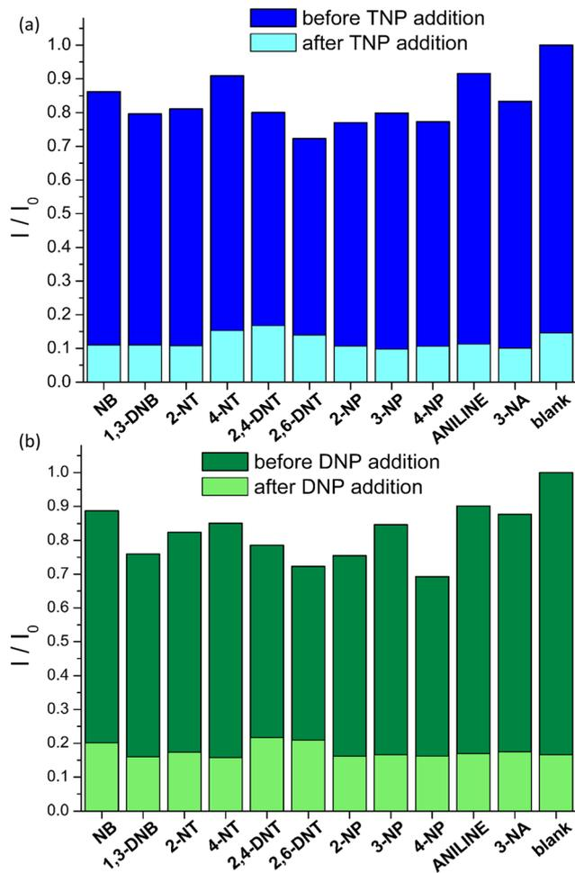
**Fig. 6** Normalized fluorescence response  $I/I_0$  ( $\lambda_{exc} = 400$  nm) of **Zr-1** suspended in H<sub>2</sub>O (2 mL, 0.1 mg mL<sup>-1</sup>) at pH 4.5 in the presence of various analytes (12  $\mu$ M). The dark bars represent the response in the presence of competing analytes and the light bars represent the response upon addition of (a) TNP (10  $\mu$ M) and (b) DNP (12  $\mu$ M).  $I_0$  corresponds to emission intensity before the addition of analytes.
