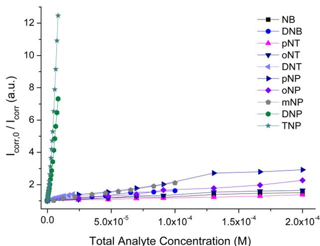
Fig. 7 Comparison of Stern–Volmer plots of fluorescence titrations ( $\lambda_{exc} = 400$  nm) of **pZr-1** suspended in  $H_2O$  (2 mL,  $0.1$  mg  $mL^{-1}$ ) at pH 4.5 with different nitroaromatic analytes.
