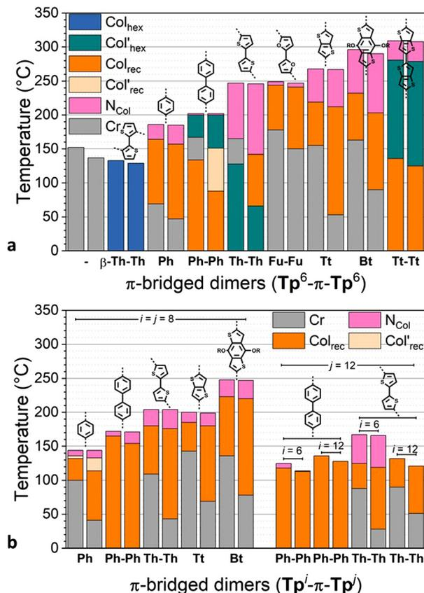
Fig. 3 Phase diagram of  $\pi$ -bridged discotic dimers (both 2nd heating and 1st cooling are displayed in bar diagram for each compound): (a)  $\text{Tp}^6\text{-}\pi\text{-Tp}^6$  and (b)  $\text{Tp}^i\text{-}\pi\text{-Tp}^j$  ( $i, j = 6, 8, 12$ ).
