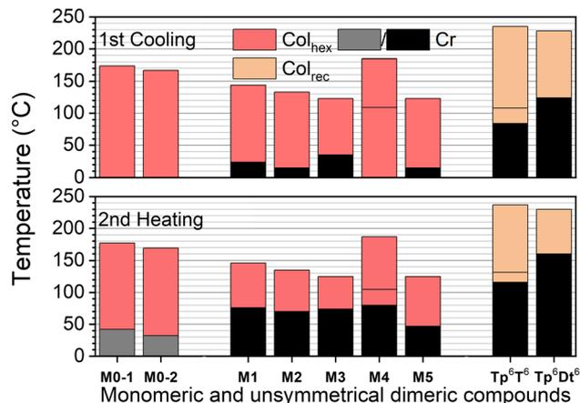
Fig. 1 Phase diagrams (top: 1st cooling; bottom: 2nd heating) of the precursors, monomeric and unsymmetrical dimeric DLCs. For **M4**, a transition between two  $\text{Col}_{\text{hex}}$  mesophases was detected by DSC and POM; For  $\text{Tp}^6\text{T}^6$ , a transition between two rectangular phases was detected by DSC and SWAXS.
