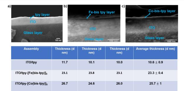
Fig. 3 (a-c) Cross-sectional FE-SEM images to deduce the thickness of electrochemically grafted ITO/tpy [Fe(bis-tpy)]<sub>5</sub> and ITO/tpy-[Co(bistpy)]5. The thicknesses from three different measurements and the average thicknesses are provided in the table for the respective layers.
