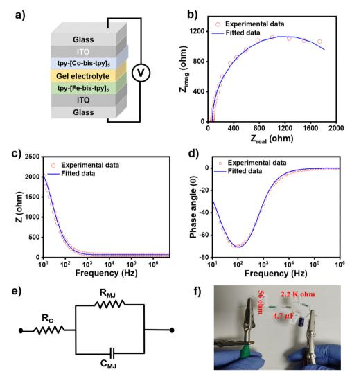
$\textbf{Fig. 7} \quad \textbf{(a) A schematic description of a molecular junction composed of ITO/tpy-[Fe(bis-tpy)]}_{5}/gel\ electrolyte/[Co(bis-tpy)]_{5}-tpy/ITO.\ \textbf{(b) The Nyquist for the property of the property of$ plot of the junction. (c and d) Bodes plot at varying frequencies. (e) The Randles equivalent circuit and f) a real circuit for the experimental validation of the fitted model.
