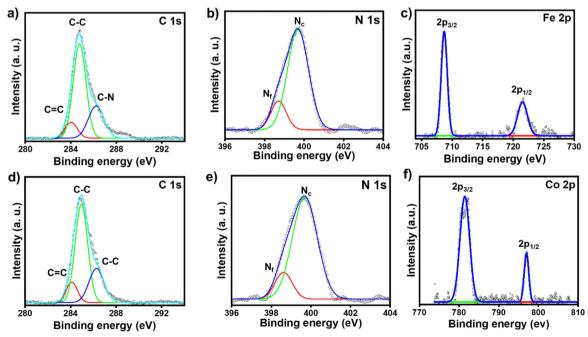
Fig. 2 (a–c) C 1s, N 1s, and Fe 2p XPS spectra of ITO/tpy-[Fe(bis-tpy)]<sub>5</sub> and (d–f) C 1s, N 1s, and Co 2p XPS spectra of ITO/tpy-[Co(bis-tpy)]<sub>5</sub>. The solid lines represent fitted data, while the open circles indicate experimental data. N<sub>f</sub> and N<sub>c</sub> stand for free nitrogen and coordinated nitrogen that binds metal ions (Fe<sup>2+</sup> or Co<sup>2+</sup>).
