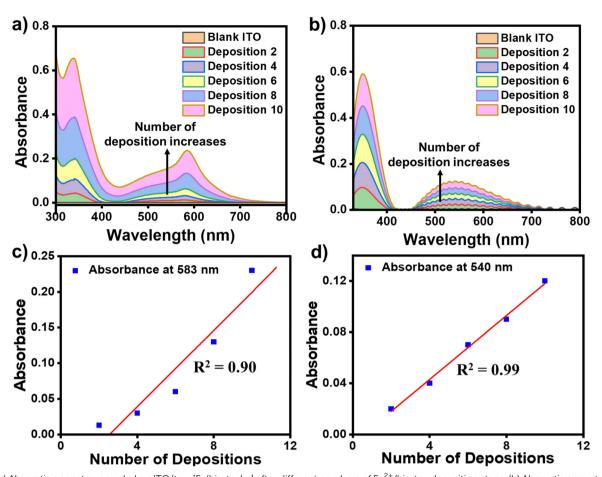
Fig. 4 (a) Absorption spectra recorded on ITO/tpy-[Fe(bis-tpy)<sub>10</sub>] after different numbers of Fe<sup>2+</sup>/bis-tpy deposition steps. (b) Absorption spectra of ITO/ tpy- $[Co(bis-tpy)_{10}]$  after different numbers of  $Co^{2+}/bis$ -tpy deposition steps. (c and d) Plots of Abs vs. no. of deposition steps for  $Fe^{2+}$ - and  $Co^{2+}$ -based molecular assemblies showing linear relationships ( $R^2 = 0.90$  and 0.99, respectively).
