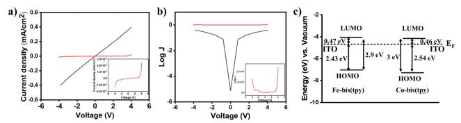
Fig. 6 (a) A comparison of the J-V plot of a reference junction (solid black line) and that of a molecular junction (solid red line). (b) Log J vs. voltage plots and (c) energy level diagrams of ITO ( $E_F$  4.7 eV) and the HOMO and LUMO energies of Fe<sup>2+</sup>-bis(tpy) and Co<sup>2+</sup>-bis(tpy).
