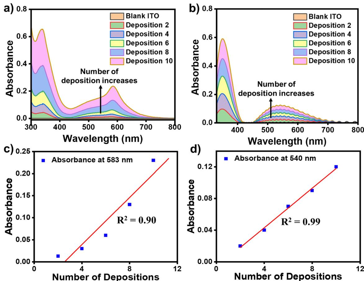
Fig. 4 (a) Absorption spectra recorded on ITO/tpy-[Fe(bis-tpy)<sub>10</sub>] after different numbers of Fe<sup>2+</sup>/bis-tpy deposition steps. (b) Absorption spectra of ITO/tpy-[Co(bis-tpy)<sub>10</sub>] after different numbers of Co<sup>2+</sup>/bis-tpy deposition steps. (c and d) Plots of Abs vs. no. of deposition steps for Fe<sup>2+</sup>- and Co<sup>2+</sup>-based molecular assemblies showing linear relationships ( $R^2 = 0.90$  and  $0.99$ , respectively).
