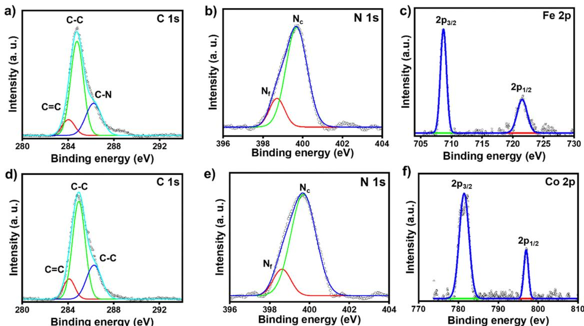
Fig. 2 (a–c) C 1s, N 1s, and Fe 2p XPS spectra of ITO/tpy-[Fe(bis-tpy)]<sub>5</sub> and (d–f) C 1s, N 1s, and Co 2p XPS spectra of ITO/tpy-[Co(bis-tpy)]<sub>5</sub>. The solid lines represent fitted data, while the open circles indicate experimental data.  $\text{N}_f$  and  $\text{N}_c$  stand for free nitrogen and coordinated nitrogen that binds metal ions ( $\text{Fe}^{2+}$  or  $\text{Co}^{2+}$ ).
