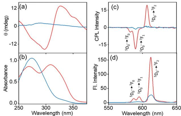
Fig. 3 (a) CD, (b) absorption, (c) CPL and (d) luminescence spectra of  $Cs^+[Eu((+)-tfac)_4]^-$  (red traces) and  $Rb^+[Eu((+)-tfac)_4]^-$  (blue traces) in chloroform (concentration = 2.0 mM; excitation wavelength  $\lambda_{ex} = 352$  nm).
