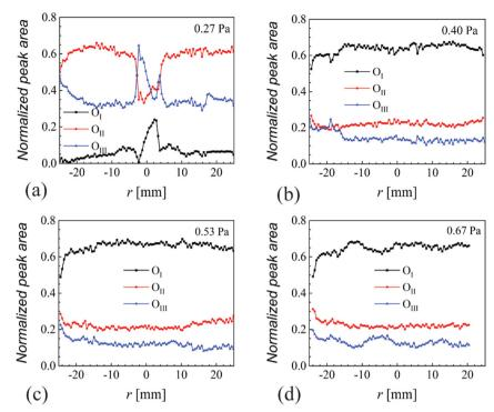
Fig. 5 Spatial distributions of the O-1s deconvolution in O<sub>I</sub>, O<sub>II</sub> and O<sub>III</sub> contributions at (a) 0.27 Pa, (b) 0.40 Pa, (c) = 0.53 Pa and (d) 0.67 Pa, respectively.
