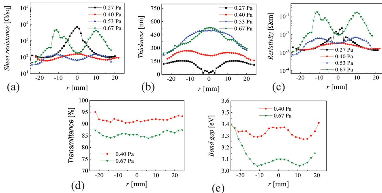
Fig. 2 Spatial distributions of the (a) sheet resistance, (b) film thickness, (c) resistivity, (d) average transmittance and (e) band gap at different discharge pressures of thin films deposited over 30 min at a 30 W RF power.
