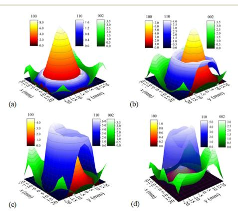
Fig. 6 2D-XRD patterns for (100), (110) and (002) orientations at (a) 0.33, (b) 0.40, (c) 0.47 and (d) 0.53 Pa, respectively.
