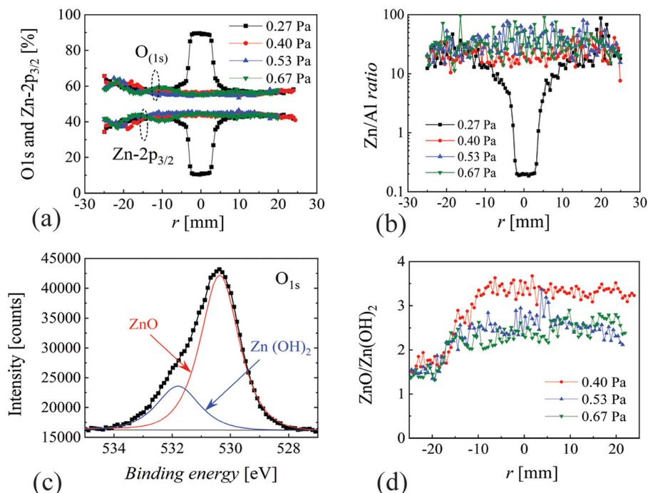
Fig. 4 XPS investigation at different pressures presenting: (a) spatial distributions of O-1s and Zn-2p<sub>3/2</sub> peaks, (b) the spatial distribution of the Zn/Al ratio, (c) O-1s deconvolution accounting for ZnO and Zn(OH)<sub>2</sub> contributions, and (d) the spatial distribution of the ZnO/Zn(OH)<sub>2</sub> ratio.
