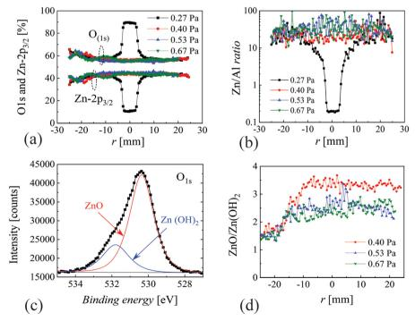
Fig. 4 XPS investigation at different pressures presenting: (a) spatial distributions of O-1s and Zn-2p<sub>3/2</sub> peaks, (b) the spatial distribution of the Zn/Al ratio, (c) O-1s deconvolution accounting for ZnO and Zn(OH)2 contributions, and (d) the spatial distribution of the ZnO/Zn(OH)2 ratio.
