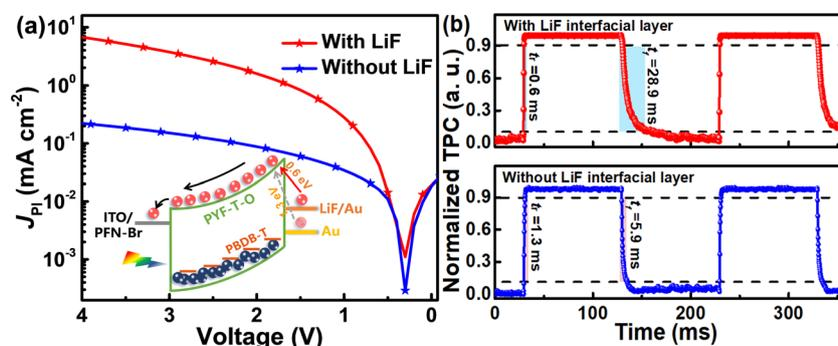
Fig. 3 PM-APDs with or without LiF layer: (a)  $J_{PI}$ - $V$  curves, the inset depicts the effect of electron injection barrier on electron tunneling-injection. (b) Normalized TPC obtained at 850 nm light-illumination with the intensity of  $1 \text{ mW cm}^{-2}$  under 4 V applied bias.
