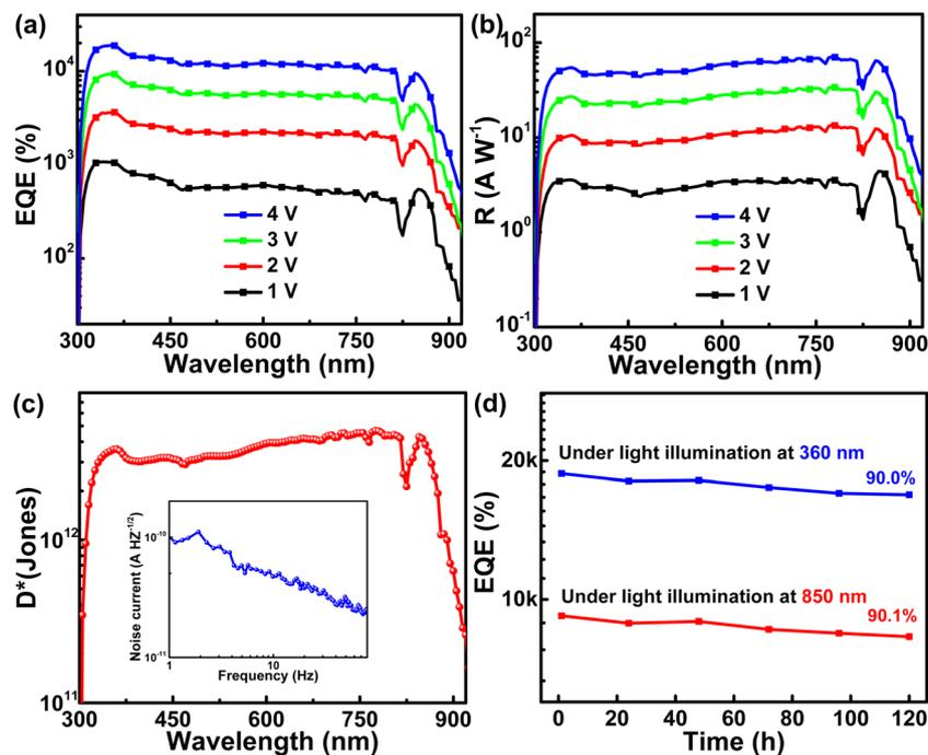
Fig. 4 Optimal PM-APDs: (a) EQE and (b)  $R$  spectra under different forward applied biases. (c)  $D^*$  spectrum and noise current under a 4 V applied bias. (d) EQE values at 360 and 850 nm under a 4 V applied bias dependent on the exposure time in a nitrogen-filled glove box.
