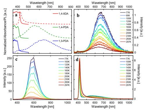
Fig. 7 (a) Absorption (solid lines) and PL (dashed lines) spectra of (1,3-PDA)PbBr<sub>4</sub> (blue line), (1,4-PDA)PbBr<sub>4</sub> (green line) and (1,4-XDA)PbBr<sub>4</sub> (red line) at 297K. (b) – (d) Temperature-dependent photoluminescence spectra of: (b) (1,3-PDA)PbBr<sub>4</sub>, (c) (1.4-PDA)PbBr<sub>4</sub>, (d) (1,4-XDA)PbBr<sub>4</sub>. All spectra are acquired using an excitation wavelength,  $\lambda_{\rm ex}$ , at 355 nm between 77 and 297 K.
