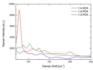
Fig. 5 Room temperature Raman spectra of (1,3-PDA)PbBr<sub>4</sub> (blue line), (1,4-PDA)PbBr<sub>4</sub> (green line) and (1,4-XDA)PbBr<sub>4</sub> (red line) excited at 632.8 nm with microscopic resolution. All the spectra are the average over 10 spectra collected along a line of 30 µm.
