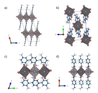
Fig. 2 Crystal structures of (a) (1,3-PDA)PbBr<sub>4</sub>, (b) (1,3-XDA)<sub>2</sub>PbBr<sub>6</sub>, (c) (1,4-PDA)PbBr<sub>4</sub>, and (d) (1,4-XDA)PbBr<sub>4</sub>.
