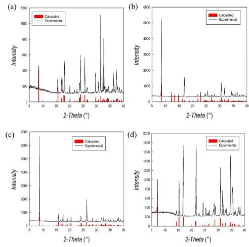
Fig. 3 XRD powder patterns of (a) (1,3-PDA)PbBr<sub>4</sub>, (b) (1,3-XDA)<sub>2</sub>PbBr<sub>6</sub>, (c) (1,4-PDA)PbBr<sub>4</sub>, (d) (1,4-XDA)PbBr<sub>4</sub> superimposed to the calculated patterns from SC-XRD (vertical red bars)
