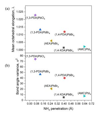
Fig. 4 (a) Octahedral elongation and (b) bond angle variance as a function of NH<sub>3</sub> penetration. PDA= phenylenediammonium; AEA = 3-(2-ammonioethyl)anilinium; XDA= xylylenediammonium; AMC = 1,4-bis(ammoniomethyl)cyclohexane. Values for (AEA)PbBr<sub>4</sub> and (1-4,AMC)PbI<sub>4</sub> are calculated from ref. 17 and 18, respectively, and their molecular structures are reported in Fig. S1 (ESI†).
