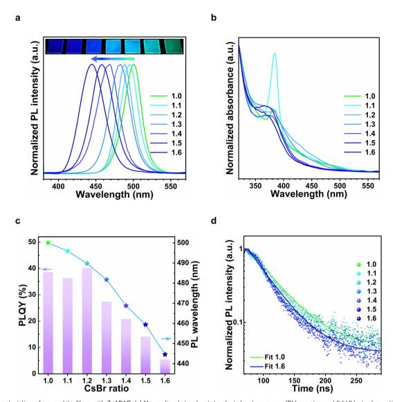
Fig. 1 Characteristics of perovskite films with 3-APAB. (a) Normalized steady-state photoluminescence (PL) spectra and (b) UV-vis absorption spectra of thin films deposited with CsBr molar ratio varying from 1.0 to 1.6 in perovskite precursors (3-APAB: CsBr: PbBr<sub>2</sub> = 1:x:1). (c) Combined PLQY and emission wavelength plots vs. CsBr molar ratio. (d) Time-resolved PL decay of perovskite samples with different CsBr molar ratio.
