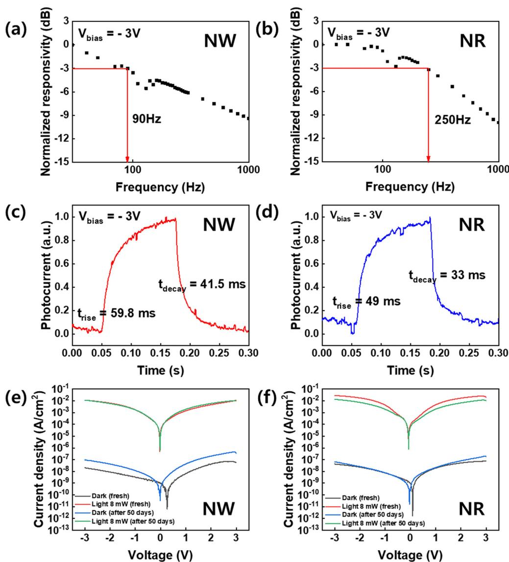
Fig. 6 Frequency responses of the CsPbBr<sub>3</sub> (a) NWs and (b) NRs photodetectors. The temporal photocurrent responses a pulse frequency of 4 Hz based on the photodetector of the CsPbBr<sub>3</sub> (c) NWs and (d) NRs. The dark and light  $J$ - $V$  characteristics of the photodetectors based on the CsPbBr<sub>3</sub> (e) NWs and (f) NRs as pristine and after 50 days.
