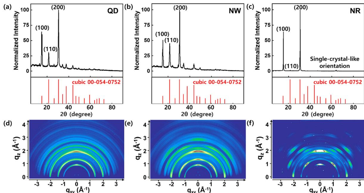
Fig. 3 XRD patterns of the CsPbBr<sub>3</sub> (a) QDs, (b) NWs, and (c) NRs with standard XRD reference (cubic: PDF 00-054-0752). 2D XRD patterns of the CsPbBr<sub>3</sub> (d) QDs, (e) NWs, and (f) NRs.
