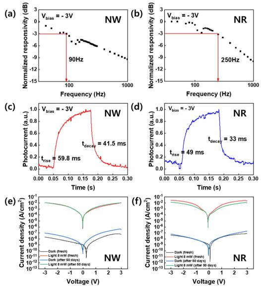
Fig. 6 Frequency responses of the CsPbBr<sub>3</sub> (a) NWs and (b) NRs photodetectors. The temporal photocurrent responses a pulse frequency of 4 Hz based on the photodetector of the  $CsPbBr_3$  (c) NWs and (d) NRs. The dark and light J-V characteristics of the photodetectors based on the  $CsPbBr_3$  (e) NWs and (f) NRs as pristine and after 50 days.
