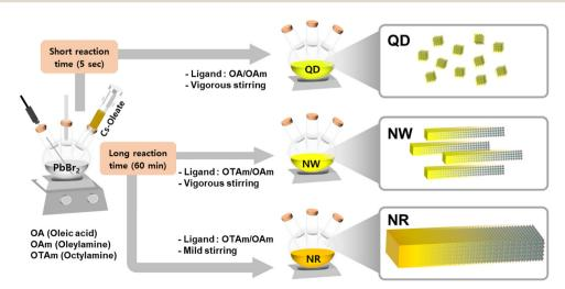
Fig. 1 Schematic illustration of the synthesis process for the CsPbBr<sub>3</sub> QDs, NWs, and NRs.
