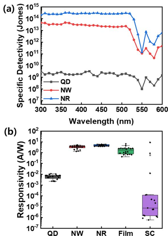
Fig. 7 (a) Specific detectivity of the CsPbBr<sub>3</sub> QDs, NWs, and NRs photo-detectors at  $-3$  V. (b) Responsivity of the CsPbBr<sub>3</sub> QDs, NWs, NRs, thin film, and single crystals (SCs) photodetectors.
