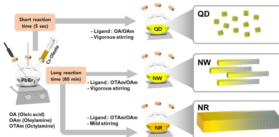
Fig. 1 Schematic illustration of the synthesis process for the CsPbBr<sub>3</sub> QDs, NWs, and NRs.
