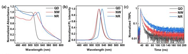
Fig. 4 (a) Optical absorption spectrum of the CsPbBr<sub>3</sub> QDs, NWs, and NRs. (b) PL spectra of the CsPbBr<sub>3</sub> QDs, NWs, and NRs. (c) Time-resolved PL decay of the CsPbBr3 QDs, NWs, and NRs with the bi-exponential fitting models.
