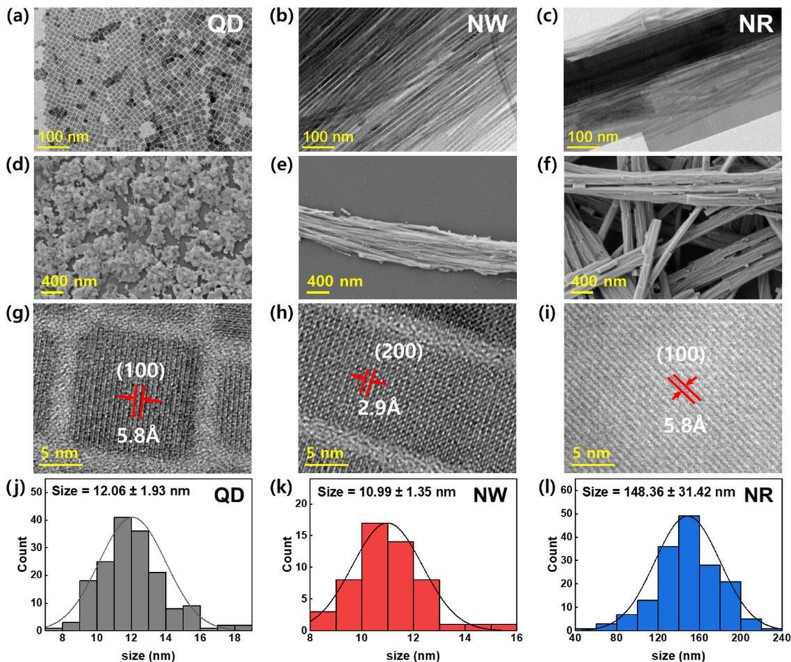
Fig. 2 TEM images of the CsPbBr<sub>3</sub> (a) QDs, (b) NWs, and (c) NRs. SEM images of the CsPbBr<sub>3</sub> (d) QDs, (e) NWs, and (f) NRs. HRTEM images with lattice fringes of the CsPbBr<sub>3</sub> (g) QDs, (h) NWs, and (i) NRs. Crystal size distribution histogram of the CsPbBr<sub>3</sub> (j) QDs, (k) NWs, and (l) NRs.
