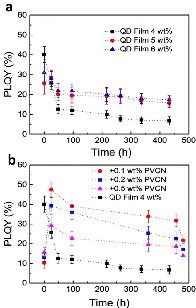
Fig. 4 Stability tests of the FAPbBr<sub>3</sub> QDs after storage under ambient conditions; the relative humidity was kept at ca. 60%. (a) Time-dependent PLQYs of neat QD films prepared using various concentrations in toluene. (b) Time-dependent PLQYs of the PeQD–PNC films; the PLQYs of a neat QD film (4 wt%) are provided to serve as a benchmark.
