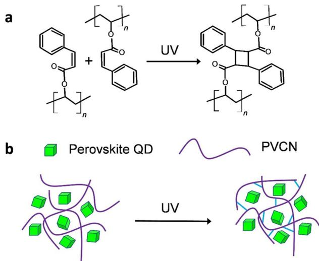
**Scheme 1** (a) Chemical structure of PVCN and its crosslinking reaction upon UV excitation. (b) Schematic representation of the formation of PeQD-PNCs based on FAPbBr<sub>3</sub> QDs and PVCN polymers, before and after UV excitation.
