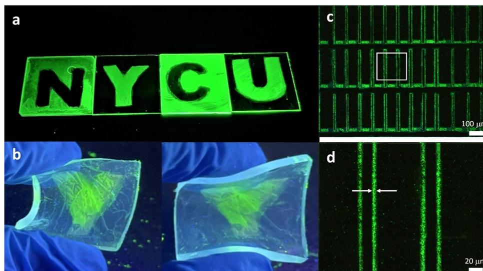
Fig. 3 Patterning of PeQD–PNC. (a) Negative patterns of the PeQD–PNC on glass substrates. (b) Pattern on a flexible PDMS substrate. (c) Microscale pattern formed using the PeQD–PNC. (d) Detailed view of the pattern, enlarged from the white square in (c).
