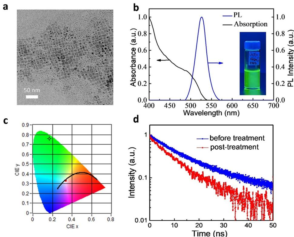
**Fig. 1** Properties of the FAPbBr<sub>3</sub> QDs. (a) The TEM image of the QDs. (b) The absorption and emission spectra of the QDs in toluene; inset: photograph of the FAPbBr<sub>3</sub> QDs in a toluene solution under UV excitation. (c) Color coordinates of the green emission from the toluene solution. (d) The TRPL decay curves of the FAPbBr<sub>3</sub> QDs in toluene.
