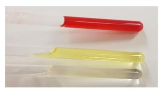
Fig. 2 Top. Donor-acceptor organogel obtained from C<sub>3</sub>NDI and C<sub>3</sub>Pyr in TCE- $d_2$  ([C<sub>3</sub>Pyr] = [C<sub>3</sub>NDI] = 5.2 mM). Middle. Solution of C<sub>3</sub>NDI in TCE (5.2 mM). Bottom. Solution of C<sub>3</sub>Pyr in TCE (5.2 mM).
