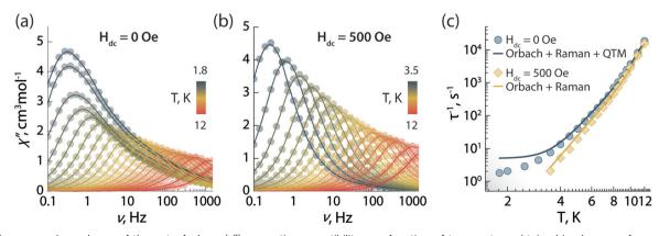
Fig. 2 Frequency dependence of the out-of-phase  $(\chi'')$  magnetic susceptibility as a function of temperature obtained in absence of an external dc magnetic field (a) and under an applied static field of 500 Oe (b). (c) Temperature dependence of the magnetic relaxation times (τ) in absence (blue circles) and in the presence of a 500 Oe applied field (yellow diamonds). Solid lines in (c) are the best fit to the experimental data using eqn (1).
