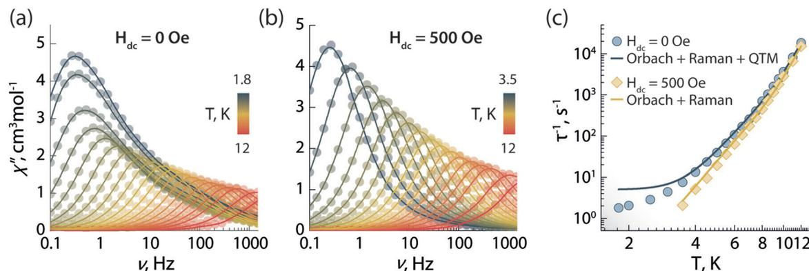
Fig. 2 Frequency dependence of the out-of-phase ( $\chi''$ ) magnetic susceptibility as a function of temperature obtained in absence of an external dc magnetic field (a) and under an applied static field of  $500 \text{ Oe}$  (b). (c) Temperature dependence of the magnetic relaxation times ( $\tau$ ) in absence (blue circles) and in the presence of a  $500 \text{ Oe}$  applied field (yellow diamonds). Solid lines in (c) are the best fit to the experimental data using eqn (1).
