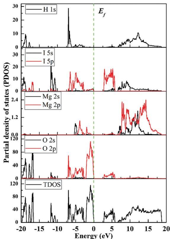
Fig. 4 Density of states for  $\text{Mg}(\text{H}_2\text{O})_6[(\text{IO}_2(\text{OH}))_2(\text{IO}_3)_2]$ .
