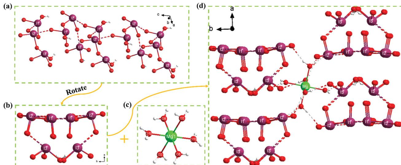
Fig. 2  $[(\text{IO}_2(\text{OH}))_2(\text{IO}_3)]^-$  infinite tubules viewed along the (a) *b*-axis and (b) *c*-axis, and the (c)  $[\text{Mg}(\text{H}_2\text{O})_6]^{2+}$  octahedron in  $\text{Mg}(\text{H}_2\text{O})_6[(\text{IO}_2(\text{OH}))_2(\text{IO}_3)]_2$ . (d) Hydrogen bonding interactions between the  $[\text{Mg}(\text{H}_2\text{O})_6]^{2+}$  octahedron and  $[(\text{IO}_2(\text{OH}))_2(\text{IO}_3)]^-$  infinite tubules.
