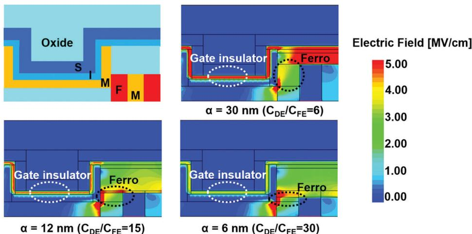
Fig. 6 Electric field profile of the 3D ferroelectric NAND flash cell during the program operation. The electric field profile of the 3D ferroelectric NAND flash cell according to the  $\alpha$  value (6, 12, 30 nm) during the program operation. The closer the color is displayed to red (blue), the stronger (weaker) the electric field intensity is. A decrease of  $\alpha$  leads to a weaker electric field across the gate insulator meaning reduced electrical stress on the gate insulator.
