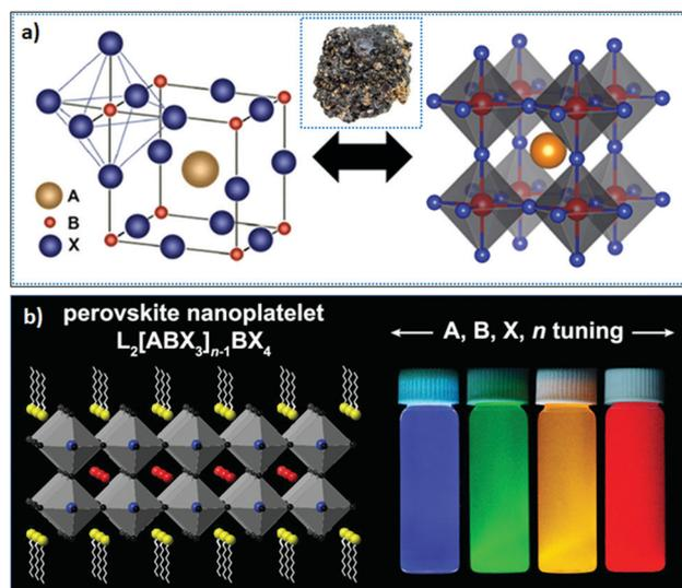
Fig. 1 (a) Bulk structure of perovskites; the inset shows the perovskite mineral CaTiO<sub>3</sub>; and (b) layered 2D perovskite ( $n = 2$ ) (left), where the emission color can be tuned upon varying X or  $n$  (right). panel (a) reprinted with permission from ref. 65. Copyright 2016 American Chemical Society. Panel (b) reprinted with permission from ref. 66 Copyright 2021 Elsevier.
