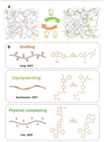
Fig. 8 (a) Schematic illustration of the strategy to complex photoswitches in the polymers; (b) schematic illustration of examples of introducing photoswitches into polymer matrix by grafting, copolymerizing and physical complexing.
