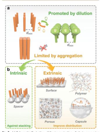
Fig. 3 (a) Schematic illustration of the isomerization of photoresponsive molecules in diluted and packed distributing states; (b) intrinsic and extrinsic strategies to improve photoisomerization in the solid state.
