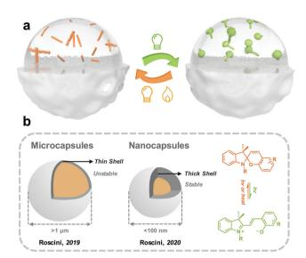
(a) Schematic illustration of the strategy to load photoswitches into the solvent-containing capsules; (b) schematic illustration of examples of reported photoswitches in solvent-containing microcapsules nanocapsules
