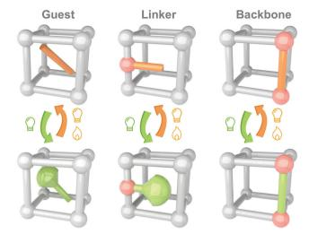
Fig. 7 Schematic illustration of the strategy to integrate photoswitches with MOFs/COFs as quest, linker and backbone
