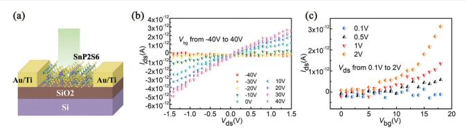
Fig. 2 Electronic properties of back-gated FETs using  $SnP_2S_6$  as the channel. (a) Schematic of the  $SnP_2S_6$  photodetector on the  $SiO_2/Si$  substrate, which provides the convenience of back gating. (b) Output curves ( $I_{ds}-V_{ds}$ ) under various  $V_{bg}$  ranging from -40 V to 40 V. (c)  $I_{ds}-V_{bg}$  curves of  $SnP_2S_6$  with different  $V_{ds}$  bias ranging from 0.1 V to 2 V.
