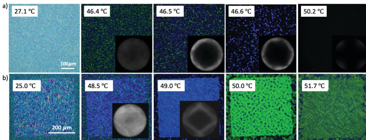
Fig. 7 Chirality Induction by the addition of chiral dopant S811 in a mixture of 13.0 wt% RM257 and BP: (a) hybrid confinement; scale bar: 100  $\mu\text{m}$ ; (b) directed self-assembly; scale bar: 200  $\mu\text{m}$ .
