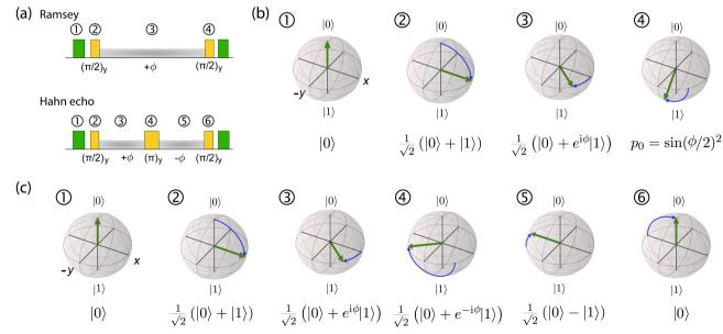
Fig. 3 Ramsey and spin-echo sensing experiments. (a) Pulse sequences for the Ramsey and the Hahn-echo protocols. Laser pulses are indicated in green, microwave manipulations are shown in yellow, and phase evolution periods are shaded in grey. (b) Bloch-sphere evolution throughout a Ramsey experiment, (c) Bloch-sphere evolution throughout a spin-echo experiment (steps 1-3 are identical to those of the Ramsey sequence).
