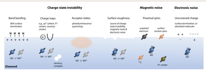
Fig. 4 Summary of sources of charge-state instability and decoherence for near-surface NV centers.
