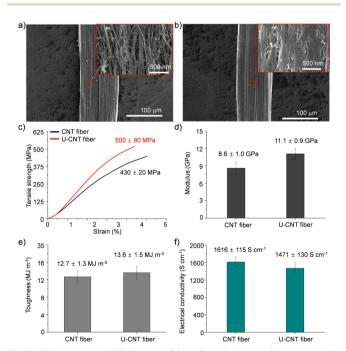
Fig. 2 SEM images of (a) CNT and (b) U-CNT fibers at different magnifications. (c) Tensile strength, (d) modulus, (e) toughness, and (f) electrical conductivity of CNT and U-CNT fibers.
