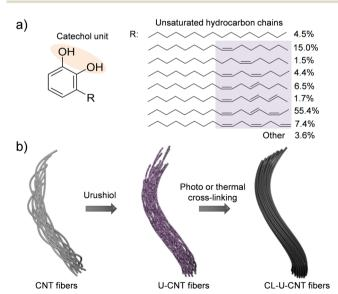
Fig. 1 (a) Chemical structure of urushiol and (b) a schematic diagram of urushiol infiltration into CNT fibers and their subsequent the photochemical and thermal cross-linking processes
