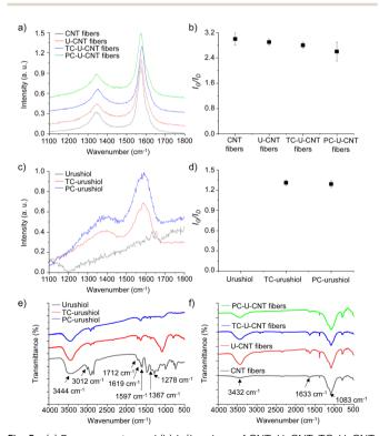
Fig. 5 (a) Raman spectra and (b)  $I_{\rm G}/I_{\rm D}$  values of CNT, U-CNT, TC-U-CNT, and PC-U-CNT fibers. (c) Raman spectra and (b)  $I_{\rm G}/I_{\rm D}$  values of urushiol, UC-urushiol, and PC-urushiol.
