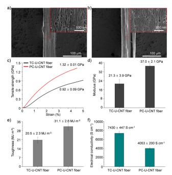
**Fig. 3** SEM images of (a) TC-U-CNT and (b) PC-U-CNT fibers. (c) Tensile strength, (d) modulus, (e) toughness, and (f) electrical conductivity of TC-U-CNT and PC-U-CNT fibers.
