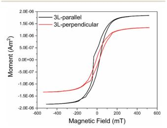
Fig. 3 MH curve at room temperature measured parallel and perpendicular to the x/y layer of the 3L samples.
