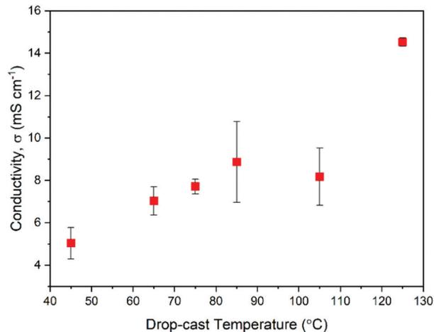
Fig. 4 Plot of thin-film conductivities of **NDI-OH** against the temperature of drop-casting used to form the film. Measurements were made at room temperature in air. Error bars were determined from film thickness measurements.
