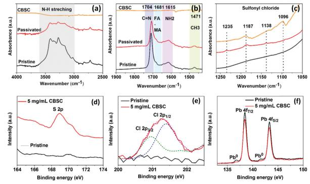
Fig. 3 (a-c) ATR-FTIR spectra of pristine, CBSC passivated and pristine CBSC films. XPS spectra of the pristine and 5 mg mL<sup>-1</sup> CBSC passivated films, specifically (d) S 2p, (e) deconvoluted Cl 2p, and (f) Pb 4f.
