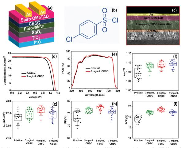
Fig. 4 (a) Device architecture of perovskite solar cells, (b) chemical structure of a CBSC molecule, and (c) cross-sectional SEM image of the CBSC passivated devices. (d) The J-V curve of the pristine and CBSC passivated devices. (e) IPCE spectra of the pristine and CBSC passivated devices. Statistical distribution of the photovoltaic parameters for all devices, specifically the (f)  $V_{\rm oc}$ , (g)  $J_{\rm sc}$ , (h) FF, and (i) PCE.
