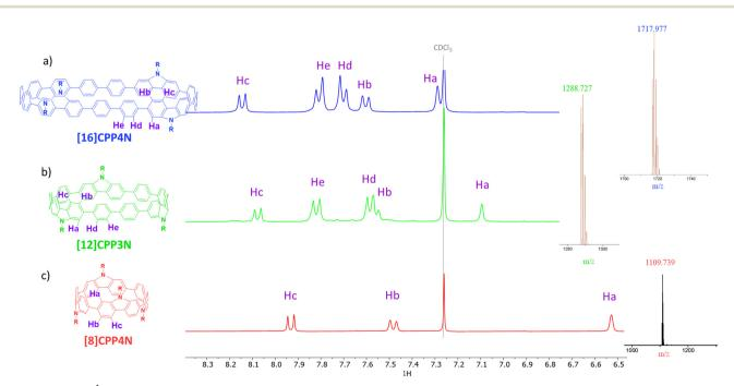
Fig. 2 Parts of the <sup>1</sup>H NMR (CDCl<sub>3</sub>) and mass spectra of (a) [16]CPP4N in blue, (b) [12]CPP3N in green and (c) [8]CPP4N in red (full spectra in ESI†).
