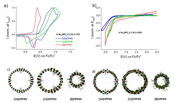
Fig. 3 Cyclic voltammograms of **[16]CPP4N** in blue, **[12]CPP3N** in green and **[8]CPP4N** in red with the Pt working electrode, sweep-rate 100 mV s<sup>-1</sup> (a) in oxidation,  $C_2H_2Cl_4 + Bu_4NPF_6$ , 0.2 M, 100 mV s<sup>-1</sup>, (b) in reduction, DMF +  $Bu_4NPF_6$ , 0.1 M, 100 mV s<sup>-1</sup> and representation of (c) the HOMO and (d) the LUMO (b3lyp, 6-31g(d), shown with an isovalue of 0.02; alkyl chains have been shortened due to calculations resources.
