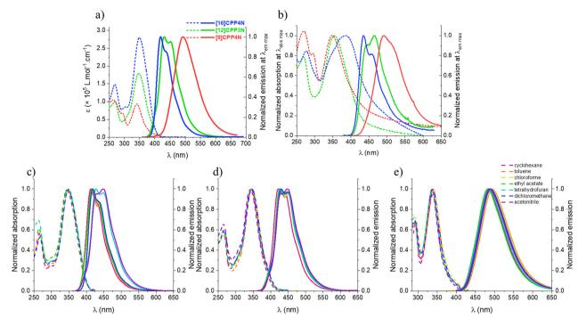
Fig. 4 Absorption (dashed line) and emission (solid line) spectra of [16]CPP4N in blue, [12]CPP3N in green and [8]CPP4N in red (a) in chloroform (b) in thin solid film (spin-coating of 1 mg mL<sup>-1</sup> solution in THF). Absorption (dashed line) and emission (solid line) spectra in cyclohexane (pink), toluene (orange), chloroform (yellow), ethyl acetate (green), tetrahydrofuran (blue), dichloromethane (dark blue), acetonitrile (purple) of (c) [16]CPP4N, (d) [12]CPP3N and (e) [8]CPP4N.
