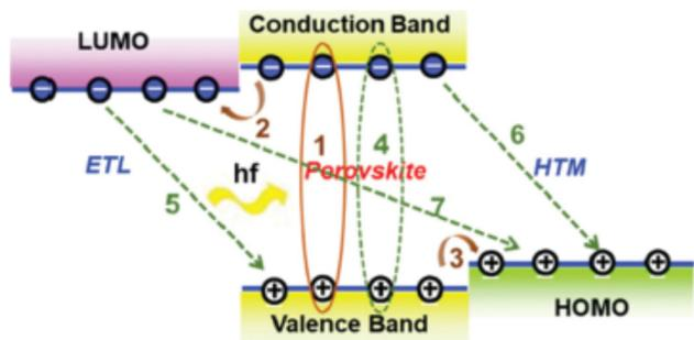
Fig. 1 Schematic diagram illustrating exciton formation upon solar illumination with photon energy  $hf$  (1), charge transfer (electron (2) and hole (3)) and recombination (4, 5, 6, 7) processes in PSCs employing both an ETL and a HTM to transport electrons and holes, respectively. Thick and thin lines, respectively, indicate processes desirable for efficient performance and recombination-induced losses. Reprinted with permission from ref. 9. Copyright 2020 Royal Society of Chemistry.
