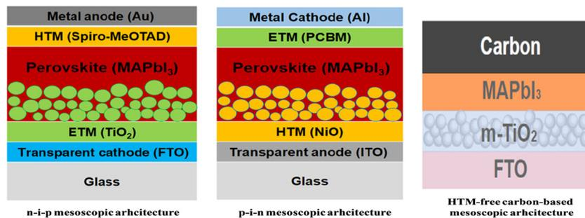
Fig. 2 Representative n-i-p, p-i-n and HTM-free carbon-based m-PSC architectures employing MAPbI<sub>3</sub> as the photoactive perovskite layer, m-TiO<sub>2</sub> as the ETL and an organic p-type small molecule (namely spiro-MeOTAD) in the n-i-p structure and m-NiO as the HTL and an organic n-type small molecule (namely PCBM) as the ETL in the p-i-n structure. Reprinted with permission from ref. 5 and 10, respectively. Copyright 2016 SPIE and Copyright 2022 Elsevier, respectively.
