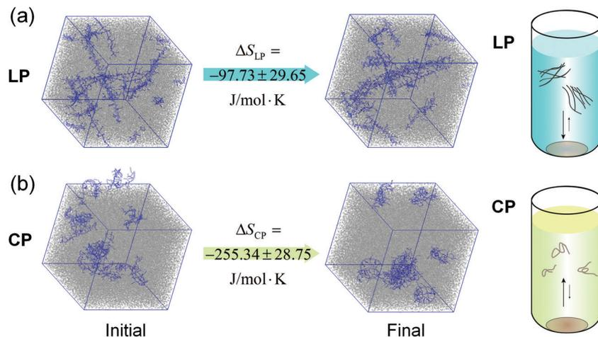
Fig. 4 Snapshots of the initial and final chain conformations of the **LP** (a) and **CP** (b) from a single simulation. The polymer chains are colored in blue and the atomic solvents are colored in gray. The entropy changes associated with the aggregation processes were shown above. An illustration of the dissolving process of the **LP** and **CP** is shown next to it.
