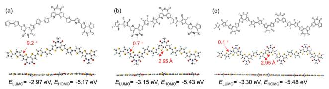
Fig. 2 Optimized molecular geometries and energy levels for (a) P(BTI-BT), (b) P(BTI-4FBT), and (c) P(BTI2-4FBT) trimers. Calculations were performed at the B3LYP/6-31G(d,p) level; the alkyl chains were replaced with methyl groups to simplify the calculations.
