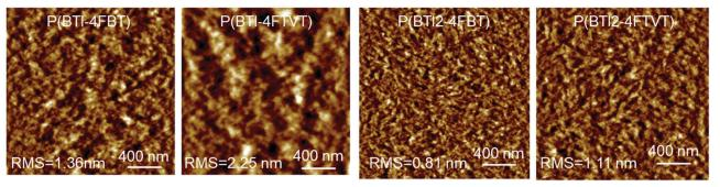
Fig. 6 Atomic force microscopy height images (2 μm × 2 μm) of polymer thin films. The films were annealed at 150 °C for 30 min in an argon atmosphere.
