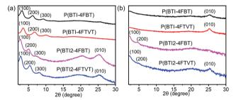
Fig. 5 (a) Out-of-plane and (b) in-plane X-ray diffraction profiles of the polymer thin films. The films were annealed at 150  $^{\circ}$ C for 30 min in an argon atmosphere.
