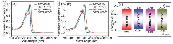
Fig. 3 (a) Solution and (b) thin-film UV-vis-NIR absorption spectra and (c) energy level diagrams of the polymers. Solution spectra were measured in o-DCB with a concentration of 10<sup>-5</sup> mol L<sup>-1</sup> of the repeating units. Thin films were prepared by spin-coating the o-DCB solutions on guartz substrates.  $E_{\text{HOMO}}$  and  $E_{\text{LUMO}}$  values were estimated from the redox onsets in the thin-film cyclic voltammetry curves.
