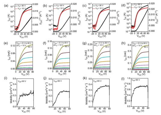
Fig. 4 Typical (a–d) transfer curves, (e–h) output curves, and (i–l) saturation mobility versus  $V_{GS}$  curves of the PEIE modified TGBC OTFT devices based on (a, e and i) P(BTI-4FBT), (b, f and j) P(BTI-4FTVT), (c, g and k) P(BTI2-4FBT), and (d, h and l) P(BTI2-4FTVT). Thin films of the polymers were prepared from o-DCB solutions and were annealed at 150 °C for 30 min in an argon atmosphere.
