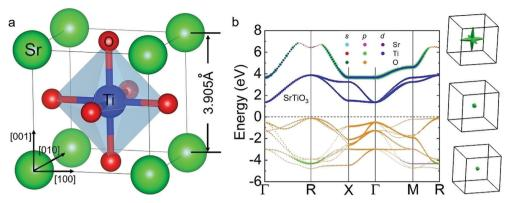
Fig. 1 Structural characterization of SrTiO<sub>3</sub>; (a) structure of the crystal and (b) the atomic orbital resolved electronic band structure. The triple degenerate CBM is located at the  $\Gamma$  point. The right panel shows the Fermi energy surface in the first-Brillouin zone with the isosurface level  $E_{CBM}+0.05$ for these three degenerate bands.
