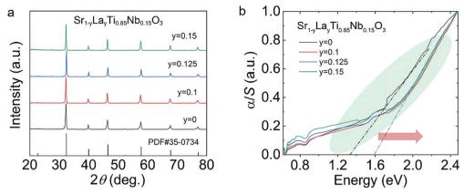
Fig. 5 Structural characterization of  $Sr_{1-v}La_vTi_{0.85}Nb_{0.15}O_3$  (y = 0-0.15): (a) XRD patterns and (b) absorption coefficient from the Kubelka-Munk method.
