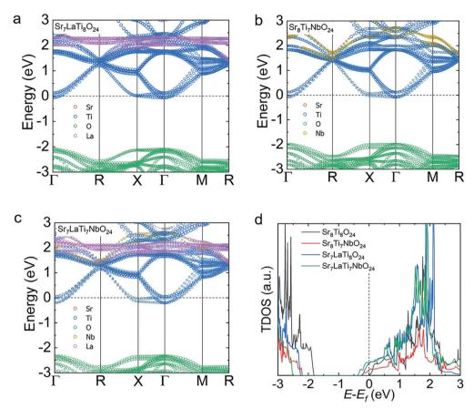
Fig. 7 Electronic band structures and TDOS calculated for the SrTiO<sub>3</sub>-based materials: (a) Sr<sub>7</sub>LaTi<sub>8</sub>O<sub>24</sub>; (b) Sr<sub>8</sub>Ti<sub>7</sub>NbO<sub>24</sub>; (c) Sr<sub>7</sub>LaTi<sub>7</sub>NbO<sub>24</sub>; and (d) TDOS near the bottom of the conduction band
