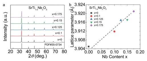
Fig. 3 SrTi<sub>1-x</sub>Nb<sub>x</sub>O<sub>3</sub> (x = 0 - 0.175): (a) XRD patterns and (b) lattice constant.
