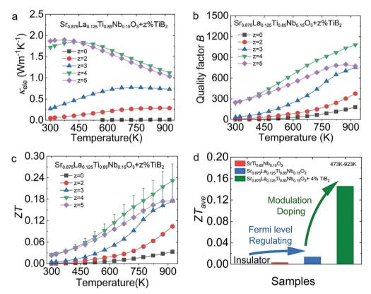
Fig. 10 Thermal transport properties of  $Sr_{0.875}La_{0.125}Ti_{0.85}Nb_{0.15}O_3 + z\%$   $TiB_2$  (z = 0-5): (a)  $\sigma$ ; (b) quality factor B; (c) ZT; and (d) average ZT of  $SrTi_{0.85}Nb_{0.15}O_3$ ,  $Sr_{0.875}La_{0.125}Ti_{0.85}Nb_{0.15}O_3$  and  $Sr_{0.875}La_{0.125}Ti_{0.85}Nb_{0.15}O_3 + 4\%$   $TiB_2$ .
