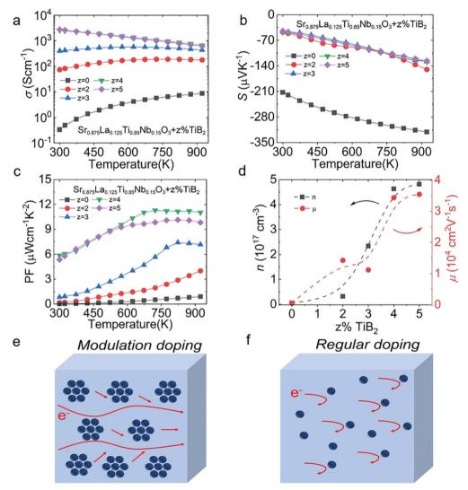
Fig. 9 Electrical transport properties for  $Sr_{0.875}La_{0.125}Ti_{0.85}Nb_{0.15}O_3 + z\%$   $TiB_2$  (z = 0-5): (a)  $\sigma$ ; (b) S; (c) PF; (d) n and  $\mu$ . (e) Modulation-doped semiconductor and (f) regular doped semiconductor.
