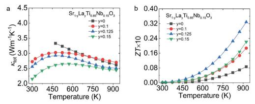
Thermoelectric transport properties of  $Sr_{1-y}La_yTi_{0.85}Nb_{0.15}O_3$  (y=0-0.15): (a)  $\kappa_{tot}$ ; (b) ZT.
