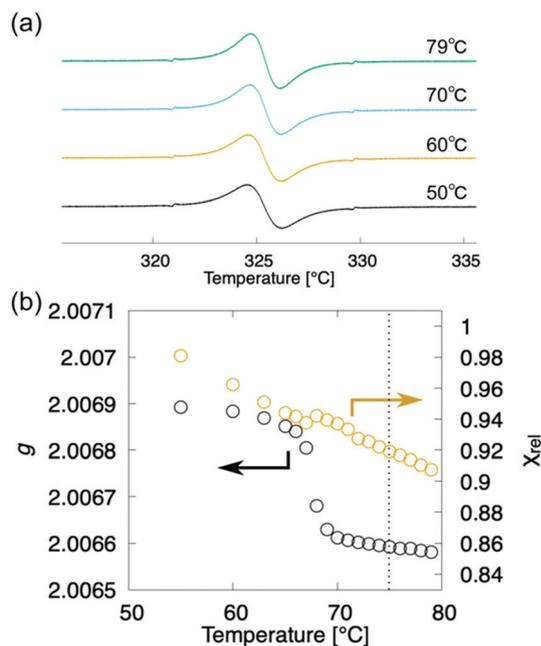
Fig. 6 EPR spectroscopy of ( $\pm$ )-**3** upon the cooling run. Black and orange circles denote the  $g$ -value and  $\chi_{rel}$ , respectively. Vertical dotted line denotes the N-to- $N_{cyb}$  phase transition point.
