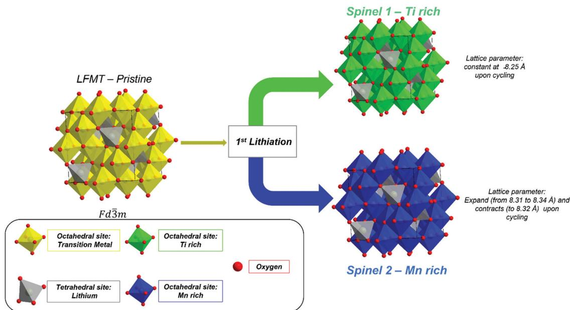
Fig. 7 Lithiation mechanism of the LFMTa-d cathodes.
