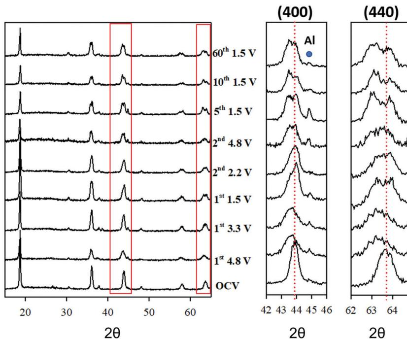
Fig. 6 *Ex situ* experimental XRD patterns during electrochemical cycling of the LFMTc cathode. The 400 and 440 reflections are highlighted in the insets. The red dotted lines refer to the peak position before cycling.
