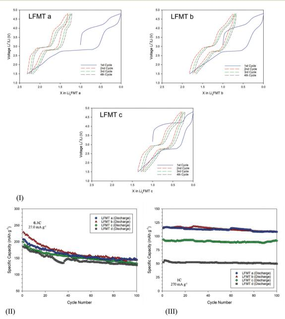
Fig. 4 (I) Voltage-composition profiles of the LFMTa-d cathodes during the first charge-discharge cycle with a voltage window 1.5-4.8 V vs. Li/Li<sup>+</sup> at C/20 rate; (II) discharge capacity upon 100 cycles at a current density of 27 mA g<sup>-1</sup> and (III) 270 mA g<sup>-1</sup>.
