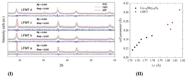
Fig. 1 (I) experimental patterns of powdered specimens collected at room temperature (empty gray circles) and corresponding calculated profile computed by Rietveld refinement (red solid line) based on cubic spinel structural model. The difference curve (blue solid line) is shown below each pattern.; (II) cell parameter of LFMT (red) compared to undoped  $Li_{1+x}Mn_{2-x}O_4$  from ref. 5 plotted as a function of the average ionic radius, i.r., of the cations
