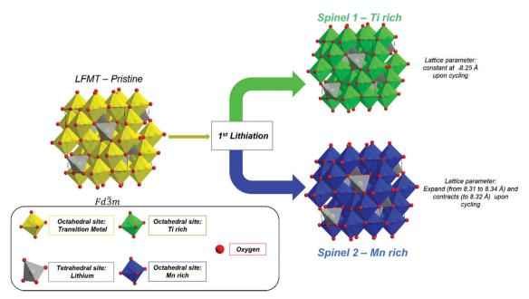
Fig. 7 Lithiation mechanism of the LFMTa-d cathodes.
