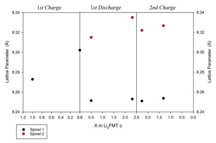
Fig. 9 Variation of the lattice parameter, a, upon cycling vs. the Li composition in the LFMTc cathode.
