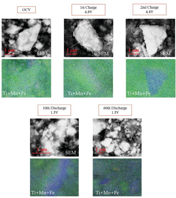
Fig. 8 SEM images and SEM-EDX maps of the LFMTc cathode before and after galavanostatic cycling. Fe (yellow); Mn (blue); Ti (green).
