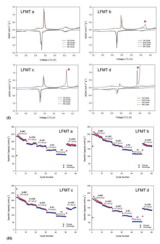
Fig. 3 (I) dQ/dV plots of LFMTa-d-based cathodes collected in the voltage range between 4.8 and 1.5 V by means of PCGA experiments at C/20; (II) rate performances of LFMTa-d cathodes cycled from 4.8 to 1.5 V at different current densities.
