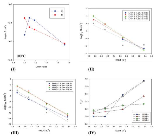
Fig. 2 (I) Ionic (red) and electronic (blue) conductivity behavior at 100 °C vs. the Li/Mn ratio; (II) Ionic and (IIIIII) electronic conductivity behavior against temperature; (IV) Li ion transport number,  $t_{1:t}$ , vs. T, for the investigated LFMTa-d active materials. In Fig. 2(II),  $\sigma_i$  values up to 100 °C are only reported for LFMTa, since the conductivity is fully electronic at higher temperature
