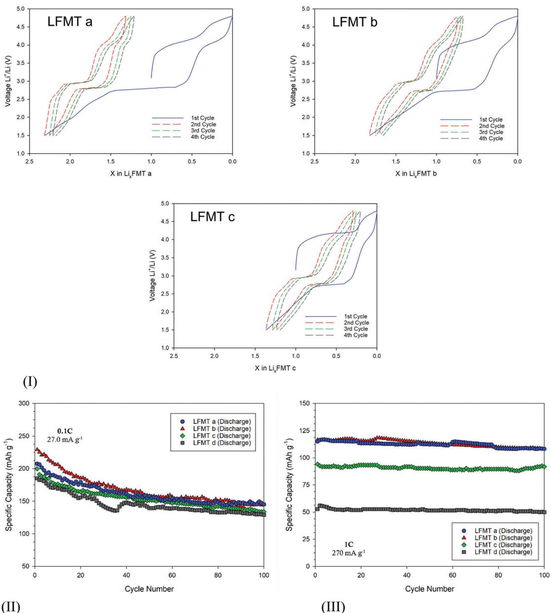
Fig. 4 (I) Voltage-composition profiles of the LFMTa–d cathodes during the first charge–discharge cycle with a voltage window 1.5–4.8 V vs.  $\text{Li}/\text{Li}^+$  at  $C/20$  rate; (II) discharge capacity upon 100 cycles at a current density of  $27 \text{ mA g}^{-1}$  and (III)  $270 \text{ mA g}^{-1}$ .
