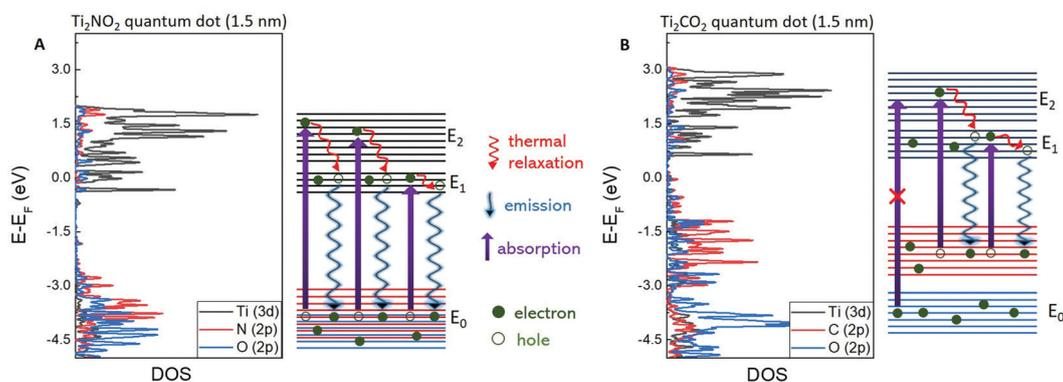
**Fig. 4** DFT calculation results of 1.5 nm  $\text{Ti}_2\text{NO}_2$  (A) and  $\text{Ti}_2\text{CO}_2$  (B) MQDs. The valence band, conduction band, and higher-energy conduction band are denoted as  $E_0$ ,  $E_1$ , and  $E_2$ , respectively.
