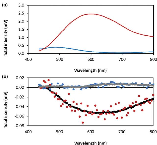
Fig. 8 (a) Total photoluminescence spectra of 6-thioguanosine at a concentration of  $30 \text{ mmol l}^{-1}$  in  $0.1 \text{ mol l}^{-1}$  of NaOH (blue) and Ag-thioguanosine hydrogel at concentration of  $30 \text{ mmol l}^{-1}$  (red). (b) CPL raw spectra of 6 independent measurements for the 6-thioguanosine (blue), the hydrogel (red), the smoothed spectrum of the 6-thioguanosine (gray) and the smoothed spectrum of the hydrogel (black).
