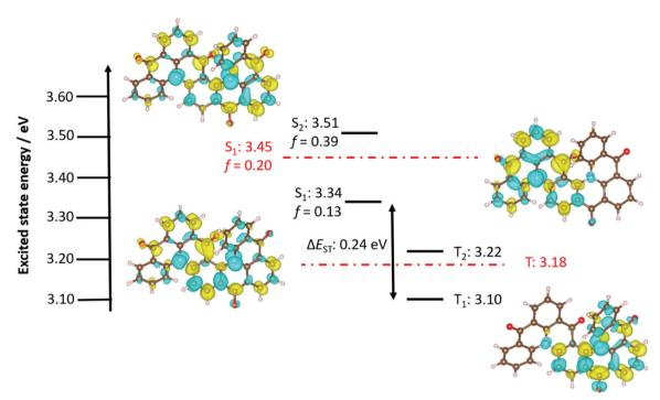
Fig. 3 Difference density plots computed at SCS-CC2/cc-pVDZ level considering only one-electronic transition contributions for (rac)-Hel-DiDiKTa. The red dashed lines show the energy levels for **DiKTa**.
