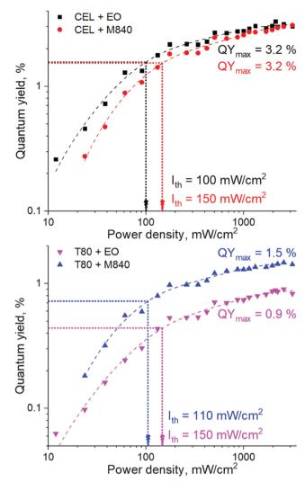
Fig. 2 Quantum yield of upconversion (QY) of CEL (top) and T80 (bottom) nanocarriers as a function of  $I_{\rm exc}$  in deoxygenated water. The dashed lines represent two-exponential fits on the data. The  $l_{\mathrm{th}}$  values were determined as the  $I_{\text{exc}}$  that yielded half of the maximum QY for each system and are indicated with the dotted arrows.
