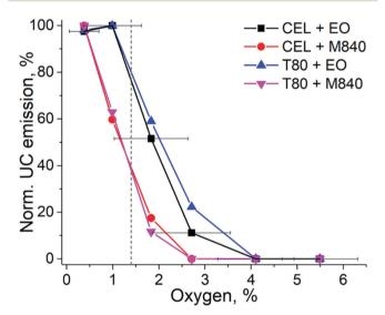
Fig. 4 UC emission intensities of each nanocarrier obtained by varying the oxygen concentration in the microfluidic chip under 140 mW cm<sup>-2</sup> excitation. The dashed grey line indicates the mean oxygen concentration (1.4%) in human tumours. The data is normalized by the highest UC intensity of each composition measured from the chip. The error bars indicate the standard deviation of oxygen % in the chip (n = 3). The oxygen levels at the used flow rates are shown in Table S2 (ESI†).
