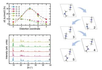
Fig. 9 MEP of transition between stable and metastable DMA+ configurations obtained from geometry optimization (top left), corresponding PXRD diffractograms (bottom left) and visualization of their structure (right).
