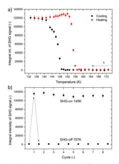
Fig. 4 (a) Plots of integral intensity of the SHG signal of DMAZn for heating and cooling cycles. (b) Plot of integral intensities of SHG signals obtained during switching experiment between 157 K and 145 K.
