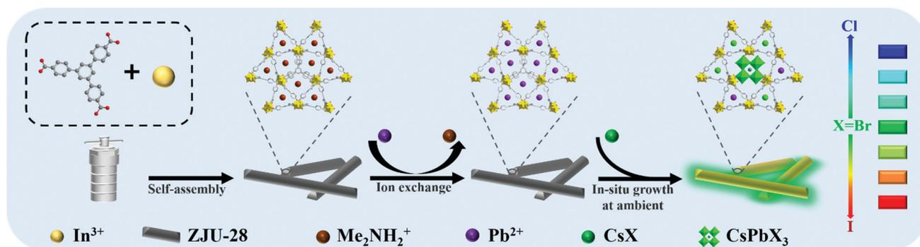
Scheme 1 Schematic diagram of the *in situ* synthesis of ZJU-28 ⊃ CsPbX<sub>3</sub> crystals with a controllable halide composition.
