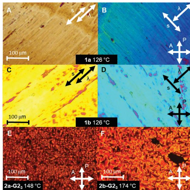
Fig. 2 POM textures under crossed polarizers. Textures of **1a** (A) and (B) and **1b** (C) and (D) after orientation by shearing with the inserted  $\lambda$ -compensation plate. The blue birefringence colour with the  $\lambda$ -plate orthogonal to the shearing direction (B) and (D) indicates that the supermesogens are oriented with their normal of the discs parallel to the column direction. Mosaic textures of 1:3 mixtures of **2a** (E) and **2b** (F) with the radical guest **G2OH**.
