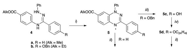
Scheme 1 Synthesis of carboxylic acids **G1OH** and **G2OH**. Reagents and conditions: (i) air, Pd/C, DBU,  $\text{CH}_2\text{Cl}_2$ , rt, overnight; (ii) KOH, THF/MeOH/ $\text{H}_2\text{O}$ , reflux, 8 h; (iii)  $\text{H}_2$  (50 psi), Pd/C, EtOH/THF, 16 h; (iv)  $\text{C}_{24}\text{H}_{49}\text{Br}$  (**6**),  $\text{K}_2\text{CO}_3$ , DMF.
