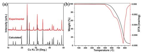
Fig. 2 (a) XRD pattern of  $Cs_2Cd_2BrCl_5$  obtained via a hydrothermal method, and (b) TG-DSC curves of  $Cs_2Cd_2BrCl_5$
