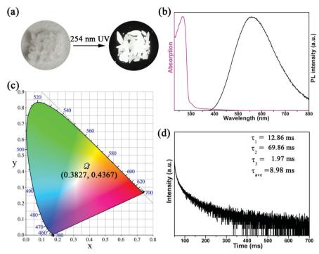
Fig. 3 PL properties of compound  $Cs_2Cd_2BrCl_5$  at room temperature: (a) images of  $Cs_2Cd_2BrCl_5$  crystals under ambient light and 254 nm UV-light excitation, (b) UV-vis absorption spectrum (purple line) and emission spectrum (black line), (c) CIE chromaticity coordinates, and (d) lifetime decay curve.
