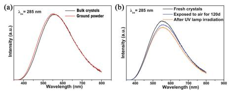
Fig. 4 (a) PL spectra of bulk crystals and ground powder for Cs<sub>2</sub>Cd<sub>2</sub>BrCl<sub>5</sub>, and (b) emission spectra of fresh Cs<sub>2</sub>Cd<sub>2</sub>BrCl<sub>5</sub> crystals, crystals exposed to air for 120 d, and after 12 h of UV-lamp irradiation.
