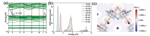
Fig. 6 (a) Cs<sub>2</sub>Cd<sub>2</sub>BrCl<sub>5</sub> band structure; (b) TDOS and PDOS, where the Fermi level (E<sub>t</sub>) is normalized to 0 eV; and (c) EDD map for Cs<sub>2</sub>Cd<sub>2</sub>BrCl<sub>5</sub>.
